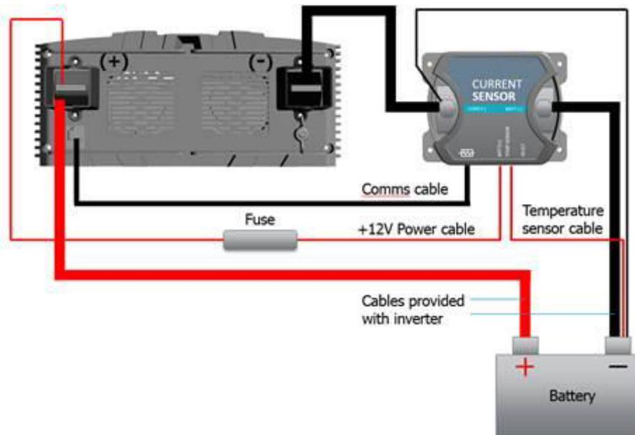
1. Using black battery cable supplied with inverter, attach one end to battery(-) terminal
